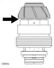
Use a thin tool to pry the deflector from the inner air cap to expose the inner air flow passages. Be very careful not to damage or distort the edges of the parts.
