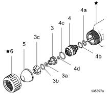
Figure 1 Round Spray Air Cap, Diffuser, and Nozzle
